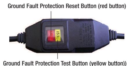
FIGURE 2 Ground Fault Protection
